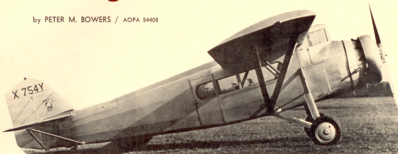
The one and only Fairchild Model 100. The name of the company changed before the airplane was ready for production, so subsequent aircraft were marketed as the Pilgrim 100. Compare fuselage and pilot's cabin lines with later models.
