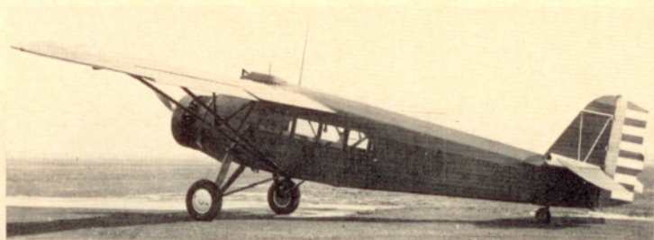
The U.S. Army bought four Pilgrims as C-24 cargo planes. Because of their Wright Cyclone engines, they are considered as Pilgrim 100-B variants when actually they incorporate features of earlier versions.
